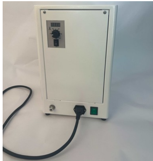
Figure 2 – Back View (Air Source, Power & Speed Control)
